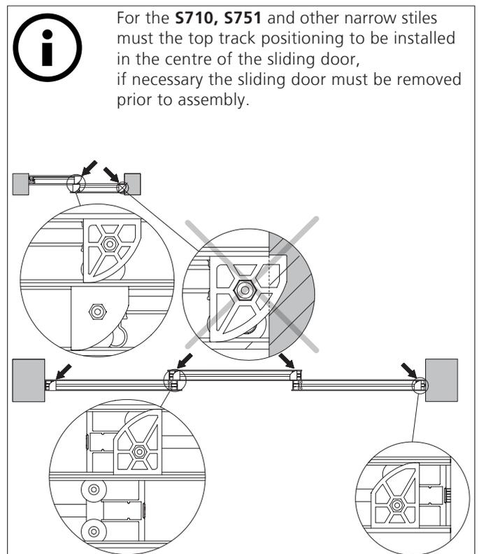
5\_ Positioning examples for the top track positioning
